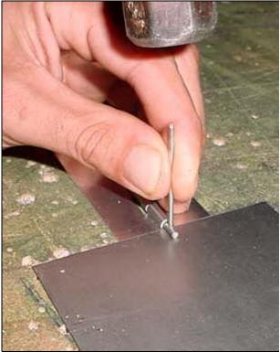
To center punch the pin: Position the stem on the pin, hammer down on the stem. Repeat the test several times, use a new stem each time.
