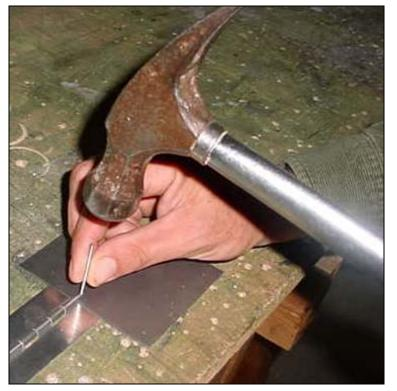
HARDNESS CHECK : Use the point on the stem from an A4 rivet to try and center punch the pin. The pin is STAINLESS STEEL if there are no scratches or impressions on the pin.
