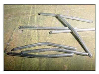
NOTE: The stem will bend on both the aluminum and stainless steel pin.
