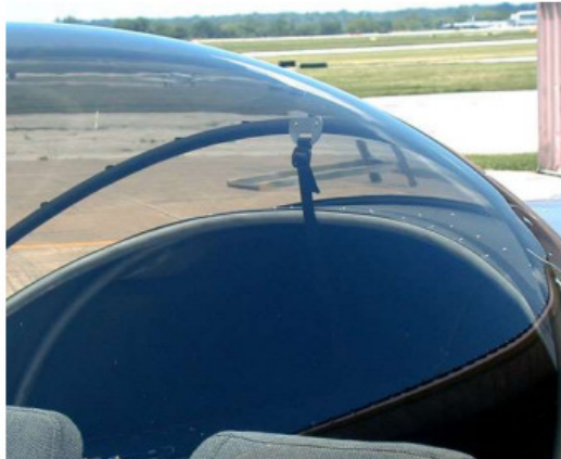
Figure 1 above: a simple strap type secondary canopy lock.
