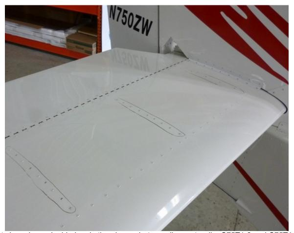
Rivets have been doubled up in the above photo on ribs centre ribs C75T1-2 and C75T1-3.
