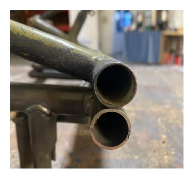
The bottom tube in the photo is thicker at 0.058". This is the correct tube type. Pedals with thinner tube must to be changed to avoid bending or possible cracking.
