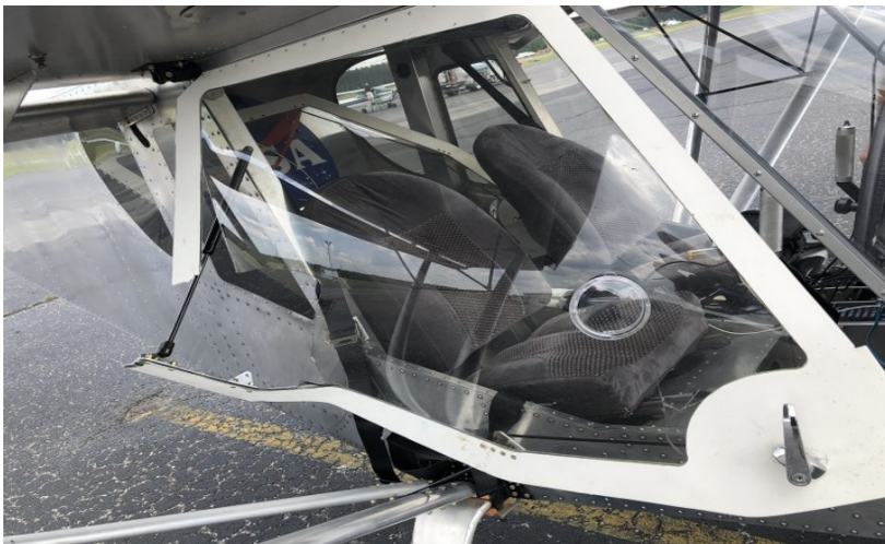
Photo shows a broken fibreglass door frame.
