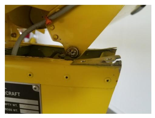
Damaged near the top hinge, easy to see after removing the top hinge bracket. When taking off or landing at an extreme angle, it is possible that the rudder can hit the ground damaging the bottom of the rudder but also the areas on the fuselage near the hinges.
