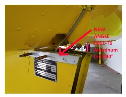
Installing new angles with 0.040" thickness and A5 rivets.
