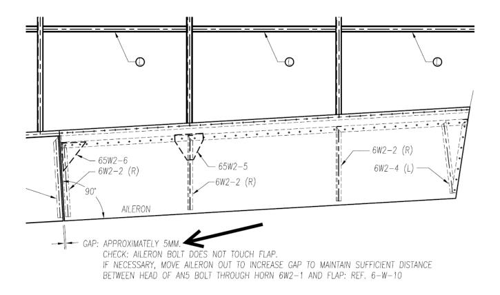
Above is from the Zodiac 650 drawings. A 5mm gap (about 3/16") is recommended between the aileron and the flap.
