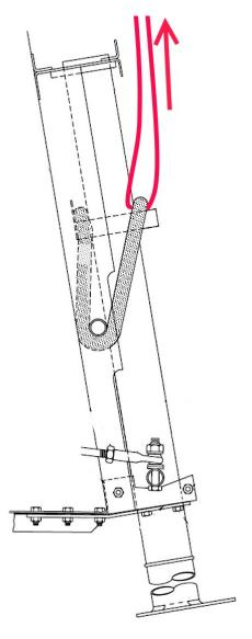
Attach the ratchet strap to an engine hoist.
