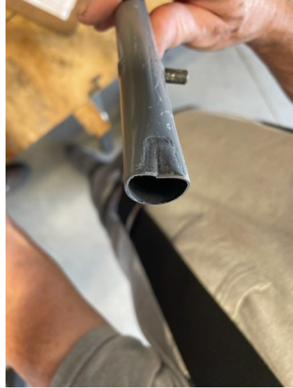
Typical damaged seat back tube, at the bottom.
