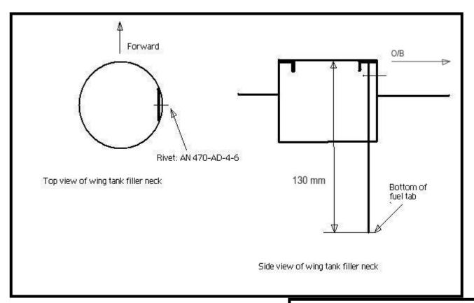
Install tab as shown in above. Install placard beside fuel filler neck. Make sure that no debris enter tanks.
