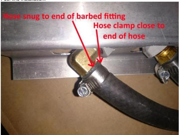
Brake and Pitot/Static line installation:
