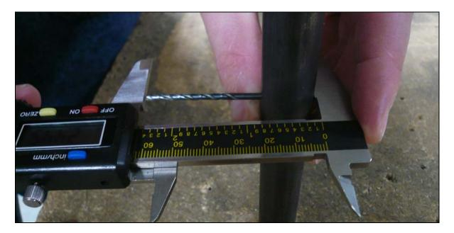
Subtract the length of the drill bit from the length of the tube and drill bit. This will tell you the wall thickness of the tube. (It is not necessary to fill the hole after drilling it.)
