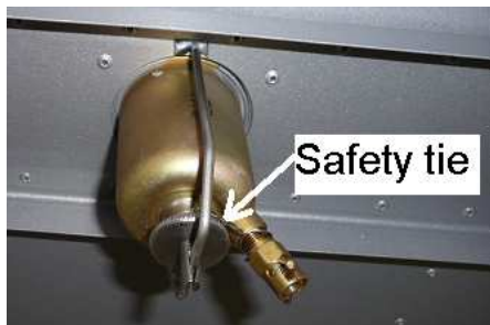
Gascolator under fuselage
