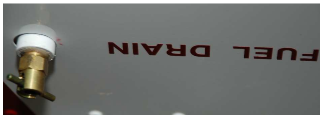
Fuel drain under each wing close to fuselage
