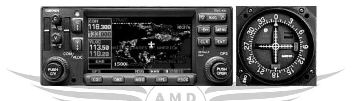
Power to the Garmin avionics is supplied from the aircraft battery to the Avionics Master Switch Breaker. Power for the Bendix/King KX155 is supplied from the aircraft power bar, through the main aircraft master.
